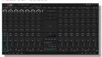
The **Dash** DSP Controller is a Windowsbased, full-featured application that configures and controls the DSP hardware. Systems can be designed to perfectly match specifications and conform as requirements change or evolve. All classes of audio processing modules for signal routing and shaping are provided.
